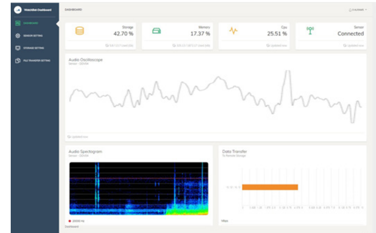
The Watchbat monitoring screen of Mobic Lab. WatchBat is a service that diagnoses failures through accurate analysis of acoustic sound data based on AI(MOVIC Lab)
